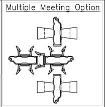
Intermediate Posts add 4" to Stack Each Lead Post adds 2-3/4" to Stack
