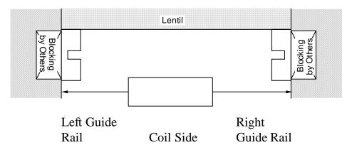
The left and right guide rails have been labeled. Position the left guide rail (making sure it is plumb) and secure it using the 3" screws provided. Attach the right guide rail making sure it is plumb and level in height with the left guide rail.
